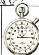
Aristo split second timer. Seven jewel movement, 1/10 second with 30 second sweep and 15 minute register. No. 102 List $80.50
